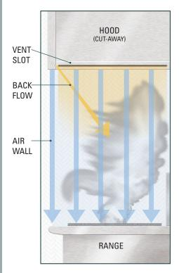
Image showing SVT smart vent technology working as smoke and effluent are created by stove. The downward air holes create a curtain keeping the smoke under the canopy while the perimeter power slot pushes the grease laden smoke toward the back of the hood into the filters.
