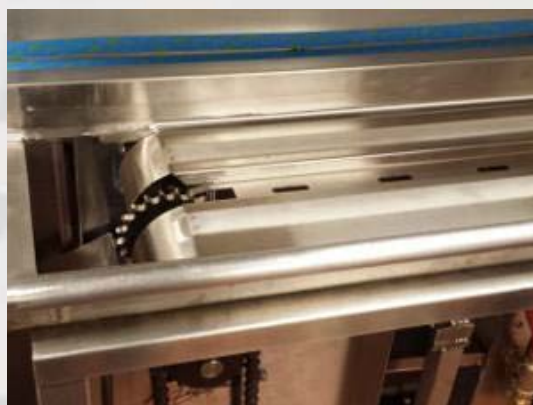
NEW BED, GEARS & BELT WASHERS
