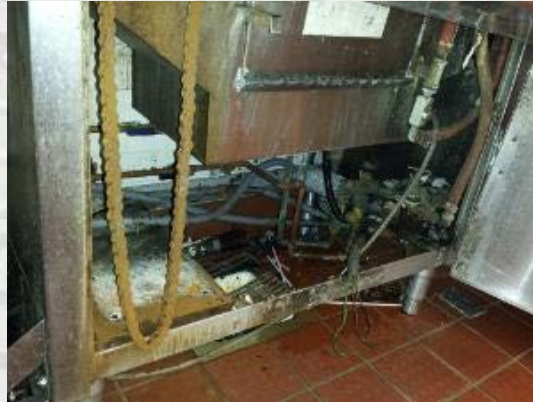
TAKING OUT THE OLD BELT WASHER
